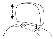
Push control to lower head restraint.
